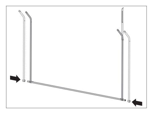
Attention: By all means, secure the table half against sliding and/or overturning for the subsequent installation steps! First, have a second person bolt the support legs attached to the table with the lateral parts.
