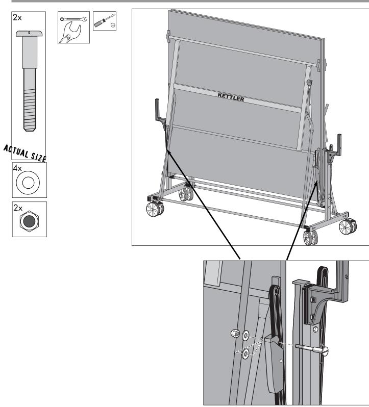
Carry out steps 6 – 8a for the second half of the table. Again, ensure that the table cannot slip or tilt over!
